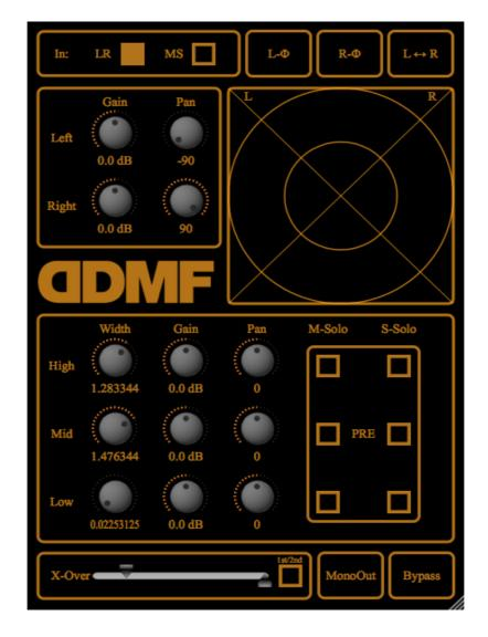
The signal chain in StereooeretS corresponds to the layout of the graphical user interface (GUI): first, the input format is specified (Left-Right or Mid-Side), which influences how the plugin interpretes the incoming audio data. Then the phases of the stereo channels can be inverted. The two channels can also be flipped. After that, the gains and stereo image positions of the left and the right channel can be adjusted independently.
