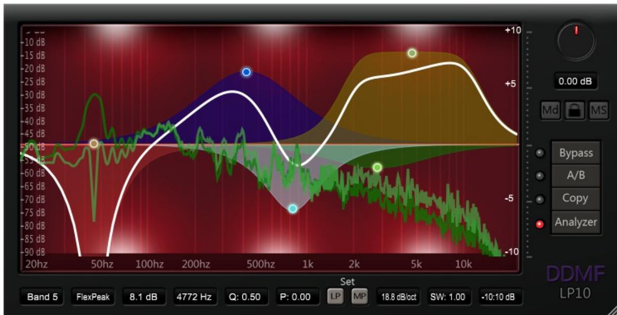
**Usage:** The LP10 is a software equalizer with up to 10 bands and 10 filter types per band to choose from. There are two ways to control the settings of the bands:
